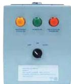
Designed to monitor and operate the backwash cleaning system, Eaton automatic control systems are simple to operate, reliable, and easily maintained. They are set to clean on differential pressure with a timed backup. The design allows field adjustments to suit the demands of the service conditions, ensuring effective cleaning with a minimum use of backwash fluid. Systems are available in automatic intermittent or continuous backwashing modes.
